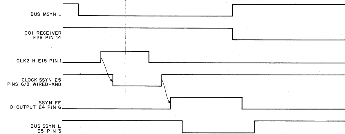
Timing Diagram for SSYN Circuit During DATO and DATOB
