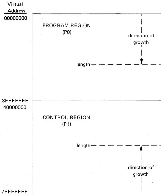
Figure 3-22 Layout of Process Virtual Address Space
