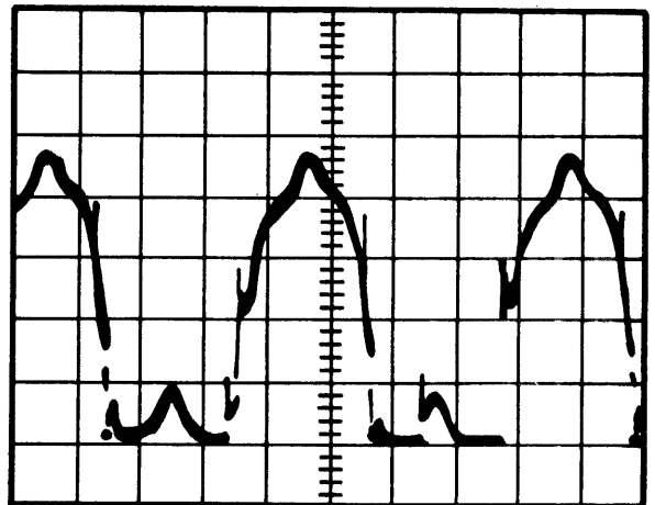
TIME SCALE: 2 MILLISECONDS PER DIVISION SPINDLE MOTOR WINDINGS LOCATION P10-6
