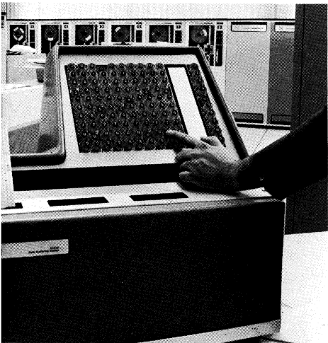
The RCA Spectra 70 Data Gathering System collects data and transmits it directly to a Spectra 70 computer or to a stand-alone controller for temporary magnetic storage—thus, providing a timely and reliable picture of business activity as it occurs.
