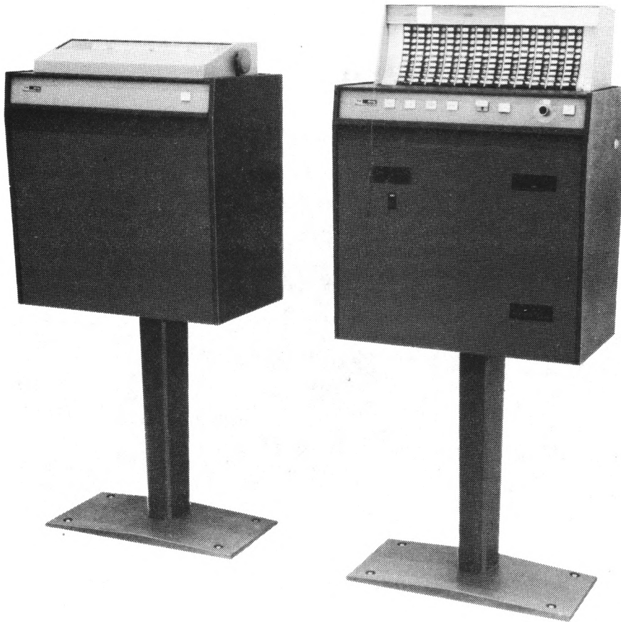
Figure 2-17. Units of an IBM 1030 Data Collection System: IBM 1033 Printer and IBM 1031 Input Station
