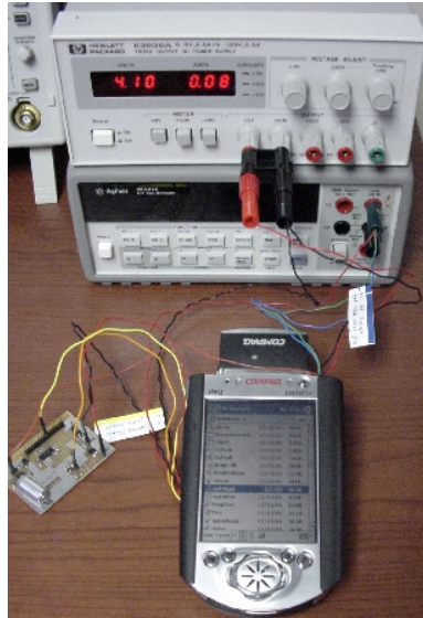
Figure 2: One of our two iPAQ prototypes showing the iPAQ handheld and PCMCIA sleeve, the energy-counter PCB, and the bench supply that powers all three.
