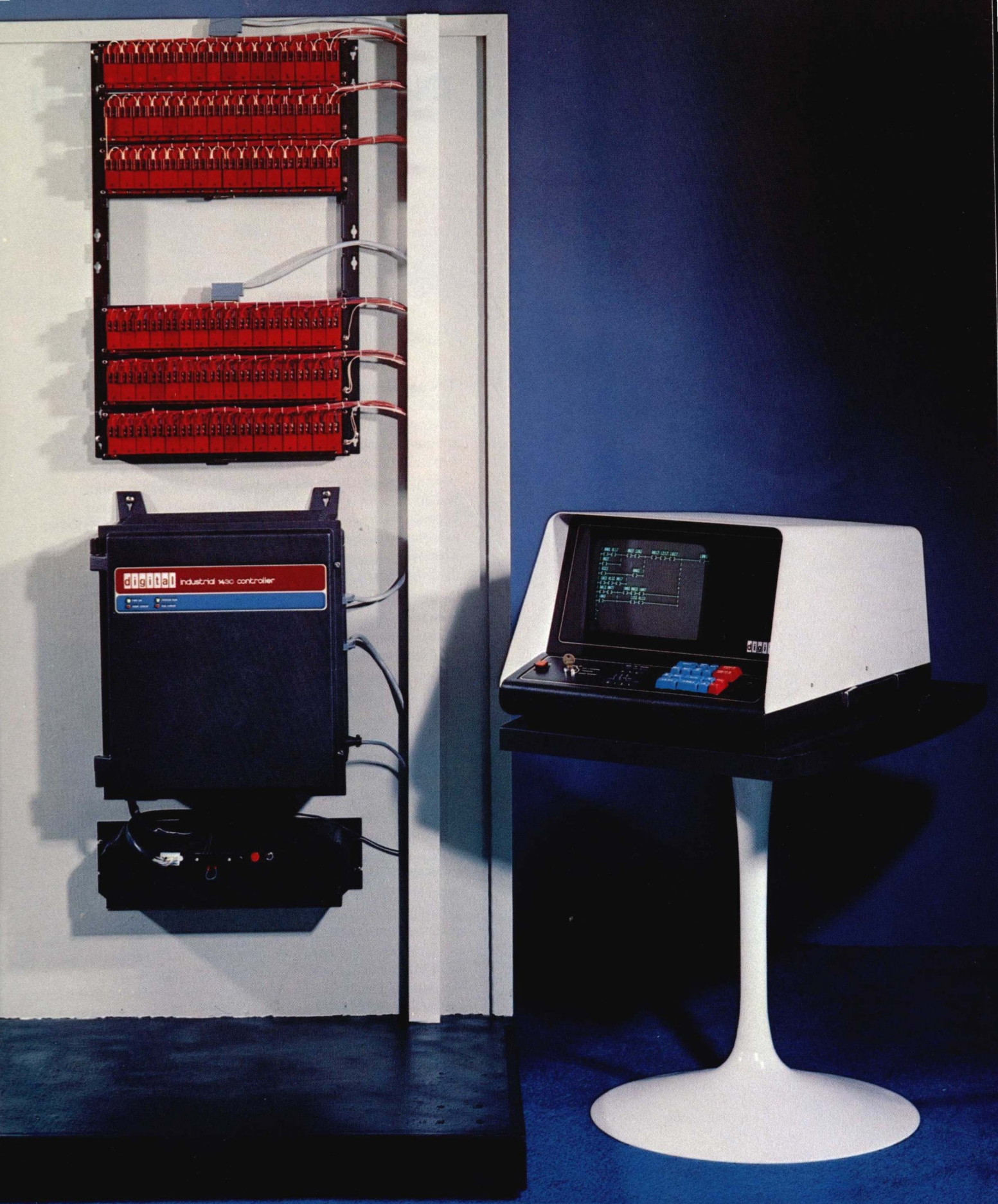
THE INDUSTRIAL 14/30 CONTROLLER WITH ITS VT14 PROGRAMMING TERMINAL
