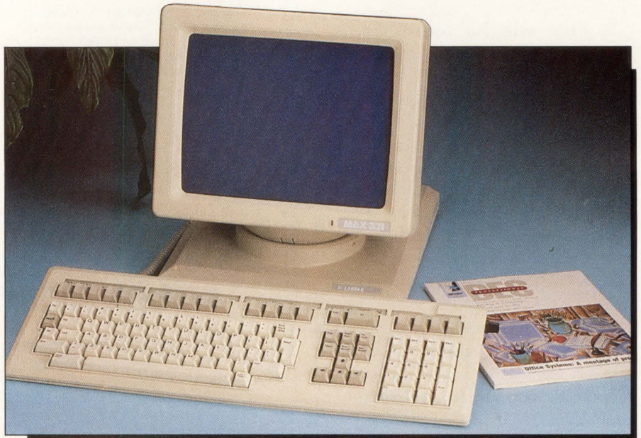
The Lanpar MAX 331 features a number of DEC emulations and can display ReGIS, SIXEL and Tektronix 4014 graphics.
