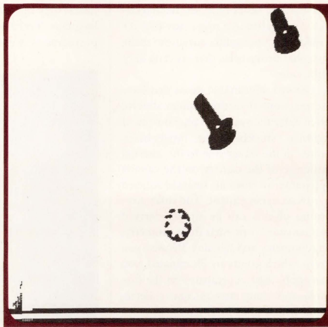
Screen 2: An example of an image subsequent to binarization. All dark regions have been set to zero and all light regions to 255 (absolute white).
