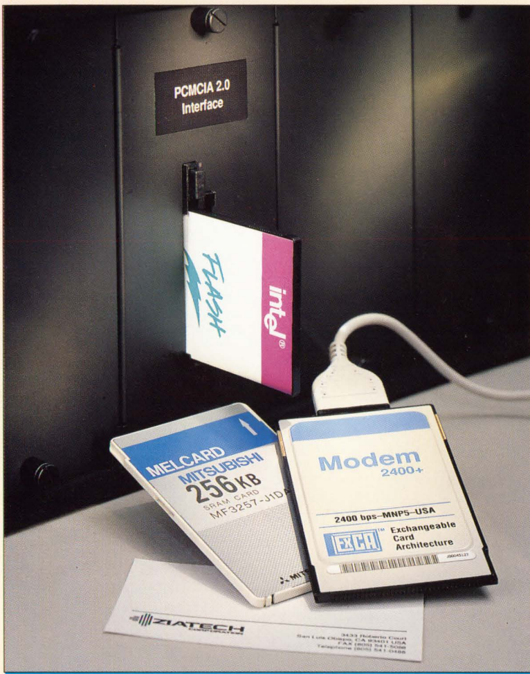
A new STD 32 interface accepts two rugged, removable, business card sized PC Card™ modules.
