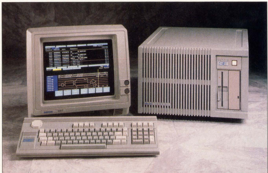
Inside this system resides Tektronix's DAS9200. The card, compatible with IEEE-896.2 profiles A, B and F, lets designers monitor high-speed timing or bus transactions on Futurebus+ systems.
