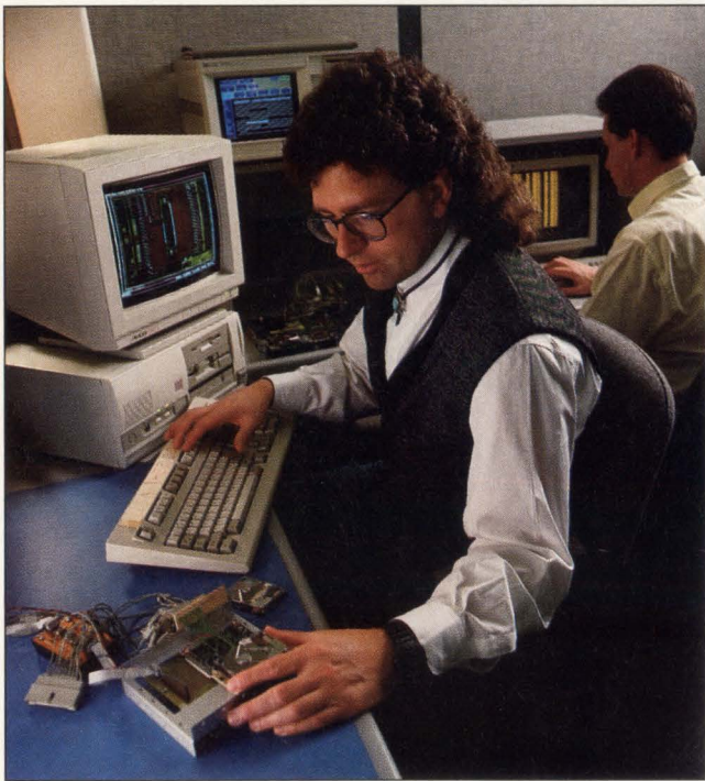
Stephen Cowen (foreground), VLSI development engineer at Integral Peripherals, and design engineer John Mount test an ASIC prototype of a 1.8-in., 20-Mbyte drive. Integral Peripherals developed its drive using half a dozen Xilinx 3042 FPGAs, and then migrated the design to an S-MOS gate array (middle chip on right side of pc board shown to the right).
