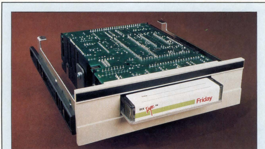
QIC-40 compatible minicartridge tape drives like Colorado Memory Systems' Jumbo use Reed-Solomon error correction to achieve error rates as low as 1 in 10^{14} bits read. This unit further ensures high reliability by integrating most drive functions into five custom ICs.
