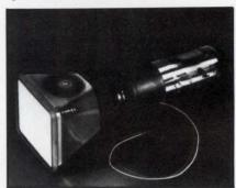
Series D14 instrument CRTs can act as compact oscilloscopes with bandwidths up to 150 MHz. These units' overall lengths measure 13.3 in. (338 mm). Optimized for CAD, the units are 5.5-in. (14-cm) post-deflection acceleration mesh tubes that deliver photographic writing speeds of 2 cm/ns. The first and final accelerating voltages of these tubes are 2.2 and 16.5 kV, respectively. Both have a 1.6 W quick-heating cathode. Amperex Electronic Corp, Providence Pike, Slatersville, RI 02876.
