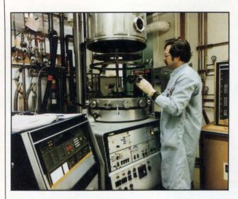
Metallization schemes are very important in GaAs processing because of the present MESFET approach. It requires a special metal alloy to be vacuum deposited directly on the ion-implanted GaAs surface. (Photo of thin-film metal deposition equipment was provided courtesy of Tektronix.)
