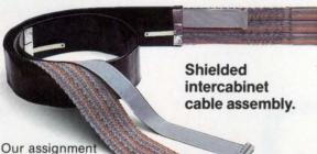
was to develop a custom interconnect cable assembly for the computer industry that met or surpassed all required FCC specifications. The solution: a Spectra-Strip 2-cable assembly consisting of a 60 conductor, 28-gauge special Twist 'N' Flat® cable with special twist length, a 26-conductor, 28-gauge Spectra GP® ground plane, 360° shielding with 2-mil aluminum mylar, wide strap drain and a 35-mil PVC jacket. Each end of both cables terminates in a MIL-C-83503-compatible socket connector.
