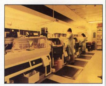
GaAs gate array processing starts in the sub-micron lithography processing area of the Tektronix GaAs foundry.
