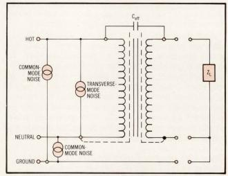
Fig 1 Ultra-isolation transformer. Two center lines represent core material or laminations.  $C_{\rm eff}$  represents effective coupling capacitance between primary and secondary coils. User equipment is protected against electrical disturbances ranges from dc to several megahertz.
