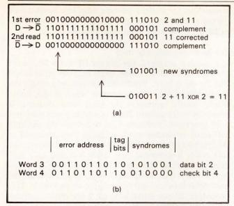
Fig 5 After correcting hard error in bit position 11 (a), system stores hard error syndrome on associative stack (b) and sets tag bit field to indicate single-bit hard error.
