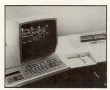
PC-800 color graphics option is provided for creating PCB artwork and associated manufacturing aids. With the option, the PC-800 operator can work with up to 7 different colors on the system's 19" (48-cm) color raster display. Up to 7 PCB layers can be simultaneously differentiated; each layer can be assigned a different color, and each color can be
