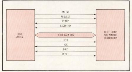
Intelligent 0.25" tape drive interface to host. Tape controller relieves host of such functions as tape formatting, data interrupt, error and file mark processing, and tape positioning. Automatic read-after-write error detecting, block buffering, and read retries are transparent to host. Should host be unable to meet streaming rate, drive will stop, reposition, and start again.
