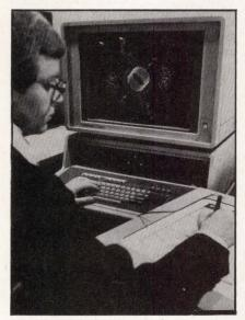
Control Data's Integrated Computer Aided Engineering and Manufacturing (ICEM) program takes users from beginning concept to finished product. Here, CD/2000, an ICEM program, is used to create a crane gear for display on the terminal screen.
