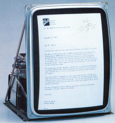
Putting over 6000 characters on a CRT display is a feat in itself. Keeping those characters crisp and stable enough to make sure all the data lines stay sharp and easily readable is even tougher. But, Ball has the answer. Our elevated line rate, regulated low voltage, and dynamic focus help provide the stability, clean alphanumeric presentation and character sharpness that will meet the toughest word processing requirements...and will keep even your most demanding customers coming back for more.
