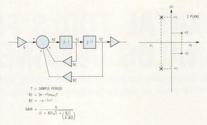
The block diagram of this filter has two delay (memory) locations (Z<sup>-1</sup>) and two feedback loops, (poles) with multipliers B1 and B2. Equations for B1 and B2 fit into the general equation for a 2-pole low pass filter.
