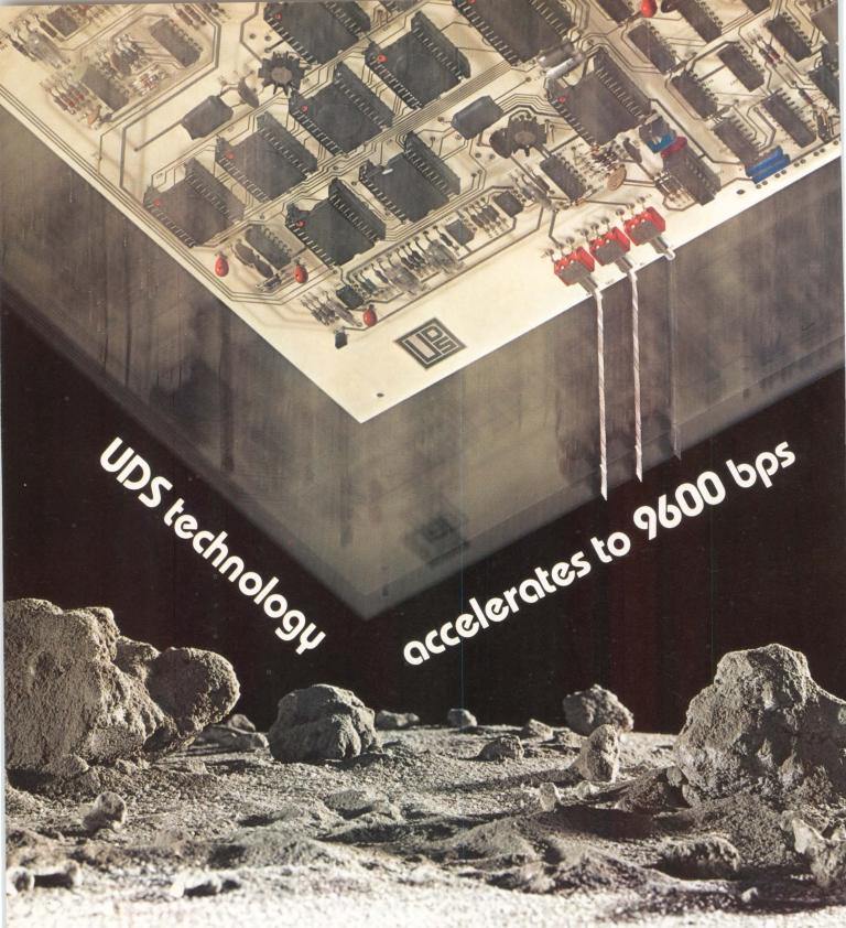
The accelerating growth in modem technology at Universal Data Systems has now produced the Company's first 9600 bps unit on a super-compact OEM board. Occupying about 100 square inches of PCB space, this microprocessor LSI modem offers dramatic space savings for designers who wish to package data sets internally in microcomputers, minicomputers or interactive terminals. The traditional UDS economy and reliability are inherent in the new 9600 bps modem.
