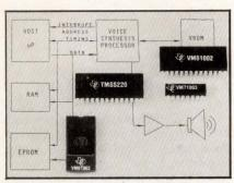
TMSK202 speech synthesis evaluation kit is used to evaluate TI's speech synthesis products for 8- and 16-bit microprocessor based systems. Voice synthesis processor can produce male, female, and children's synthesized speech as well as variety of sound effects. EPROM and two VROMs store total of 256 words, phrases and sounds. These can be linked together by user and output to amplifier as synthesized speech.
