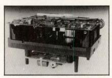
The Super Sidewinder 45M-byte (formatted) 0.25" streaming cartridge tape drive with a transfer rate of 90k bytes/s provides 8" and 14" Winchester backup at \$20/M byte. Manufactured by Archive Corp, it can back up 160M bytes in 33 min with three media changes. Two models are available: basic and intelligent. Both provide high streaming at 90 ips and eliminate the inter-record gaps associated with traditional start/stop tapes. The drives use a serpentine re-
