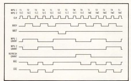
Fig 4 Dual processor bus timing diagram. Wait states are inserted when necessary to allow slower system elements and procedures to catch up with processors.
