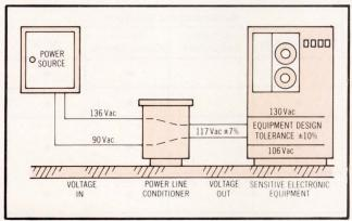
Fig 3 Power line conditioner application. Varying input voltages, as low as 90 Vac and as high as 136 Vac, are received and immediately regulated to within  $\pm\,7\%$  of nominal. Thus, ac power is controlled within the  $\pm\,10\%$  design limits of most sensitive equipment. Noise attenuation is also provided by its ultra-isolation transformer to protect against noise and transients in ac power source.
