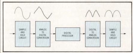
Fig 1 Converting analog signals to digital data. Processor chips convert input analog signals to digital data through A-D conversion, while analog outputs are sent through D-A converter.
