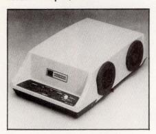
Microprocessor controlled AJ 1233 communicates with Bell 212 and 103/113 VA 3400, and AJ 1200 series modems. It is switch-selectable for communications at data rates of 1200 bps synchronously or asynchronously, and from 0 to 450 bps asynchronously. The device can be used in all modes either as an acoustic coupler or modem, directly connected to the switched network by a modular RJ-11C
