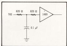
The RS-232 drivers in the SSM AIO card are the same as Pearson's Fig 2. At 1200 baud the input filter integrated the signal to the extent that the voltage swings at the 1489 barely exceeded the standard  $\pm$  3-V thresholds at the extreme peaks. The transition times (see Pearson's Fig 1) were the same as the bit length at 1200 baud—much greater than 0.04  $T_{\rm PD}$ . For driving true RS-232 inputs with cables there is nothing wrong with the circuit shown in Pearson's Fig 2, but it
