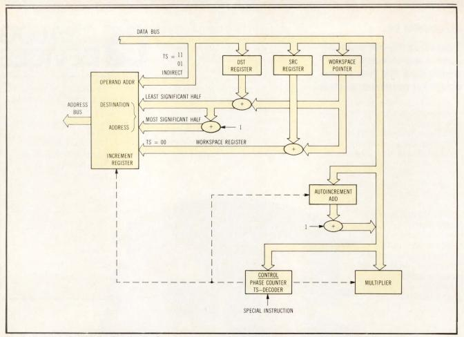
Fig 2 Functional multiplication circuit. Activated when special instruction signal is sent from special instruction switching unit, control unit decodes addressing mode and actuates phase counter. Workspace registers are updated by means of routine 1/0 instructions or by direct decoding of two instructions affecting registers.
