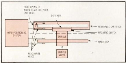
Fig 1 Cross-section of DMA System's Micro-Magnum fixed/removable drive. 0.75" (1.9 cm) high cartridge is removable medium for system 1/0 and file backup. Removable cartridge and drive compartment are automatically sealed. Servo information is embedded on disk, providing reliable cartridge interchange.
