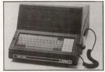
Enabling new or existing computer systems to use bar coding for data collection and management, Series 7 terminal allows 2-way (full-duplex) communication between a mainframe and any number of remote workstations. It features a full alphanumeric keyboard, handheld stainless steel bar code scanner with either an infrared or red LED light source, 32-char dot matrix display, and
