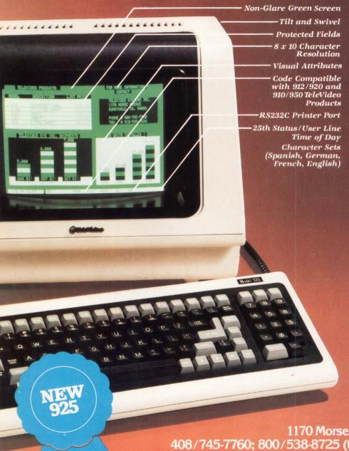
Now you can have it all with TeleVideo's new 925. Code compatible with our 910 and 950 terminals, the 925, with its 6502 microprocessor-based control board can emulate our 912/920 models while operating at speeds up to 19.2K baud. This allows you to grow within the TeleVideo family of terminals, from the conversational to the smart.
