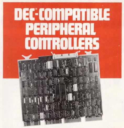
Dataram Corporation offers the industry's widest range of DEC-compatible peripheral controllers — from comparatively simple NRZI tape controllers to complex 300 MB storage module drive (SMD) controllers.
