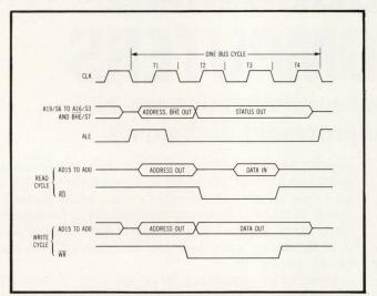
Fig 1 Timing diagram for 8086 microprocessor. Since at least four timing states (800  $\mu$ s at 5 MHz) are required for each bus transaction, typical RAM chip operates at half speed when used in conjunction with single 8086 processor.
