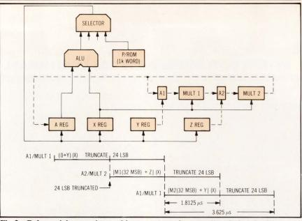
Fig 3 Polynomial expansion architecture. EAU elements directly involved in polynomial expansion process are dual, serial, and overlapped adder/multipliers. Architecture is controlled by command word sequences, and each machine cycle by one command.
