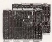
Q-bus embedded dual-density tape controller.
