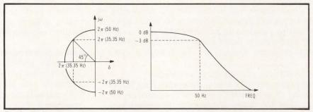
Fig 2 Butterworth filter complex pole relationships and associated attenuation curve. Circle represents filter cutoff frequency (50 Hz) with 45° pole locations coinciding with -3 db points.
