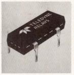
Teledyne's 640-1 is a solid state pin compatible replacement for DIP reed relays where higher reliability and long life are required. Switches AC or DC up to 50V. Low on-resistance is 2 ohms. Control voltage range is 3.8 to 10VDC. Transformer coupling provides 1500(P-P) isolation, low off-state leakage, & high switching speed. Employs hybrid microcircuits in TO-116 DIP. \$6.15 ea for 5000 pcs. TELEDYNE RELAYS, 12525 Daphne Ave, Hawthorne, CA 90250. Tel: (213)777-0077 CIRCLE 476
