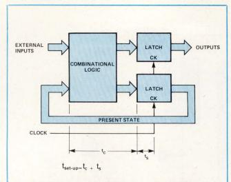
Fig 4 State machine setup time. When interfacing synchronous state machine with asynchronous switch matrix, total setup time must reflect both propagation delay of combinatorial logic and setup time of latch
