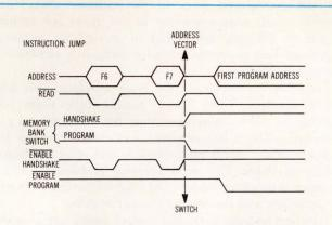
Fig 3 Memory bank switching. Microprocessor access to last restart instruction (F7, program starting address vector) initiates switching from handshake memory to program memory. Switching occurs on trailing edge of READ to avoid race condition
