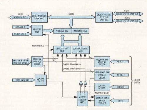
Fig 2 Universal interface block diagram. Multiplexers give either object microprocessor or host computer access to shared memory. Control register determines which of these gains memory access. Memory bank switch latch is key to microprocessor transparent operating system
