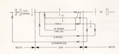
Fig 1 Stop and wait protocol. Transmitter must wait for ACK, NAK, or time-out before sending data block
