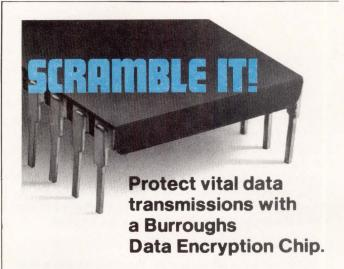
Build data security into point-to-point or multipoint communication networks. This encryption/decryption chip uses the National Bureau of Standards Data Encryption Standard (DES) algorithm to encrypt or decrypt eight bit bytes of data per encryption cycle. Encryption is based on a 56-bit key variable which cannot be accessed once it is loaded in the key register of the chip.
