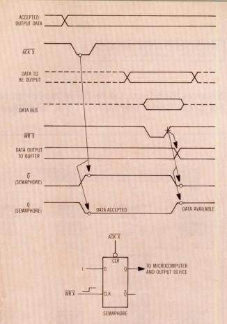
Fig 3 Conditional output with semaphore. Sequence of timing signals and data transfers are demonstrated by timing diagrams for microcomputer output using semaphore
