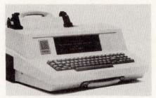
Easy to use Findex system employs BASIC language operating system for handling general business, as well as engineering, functions. Small unit stores 128k bytes of data in magnetic bubble memory. Printer and plasma display round out the package
