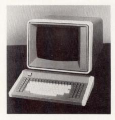
Satellite display terminal 850 includes up to 8k of P/ROM for programming and 4k or 16k of RAM for buffer and screen storage; 4k bits of EAROM are optional. Features of the intelligent standalone terminal include a separate current loop that enables the terminal to assume receive functions of a Telex machine, pass words, telephone numbers, and delimiters. The 15" (38-cm) screen has a display format of 80 char by 25 lines. **Megadata Corp**, 35 Orville Dr, Bohemia, NY 11716.
