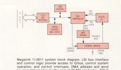
count registers allow buffer area of 32,767 words max. SDLC controller hardware performs data encoding and decoding, address checking, and error checking. Digital PLL recovers receive clock from data stream to time data into registers
