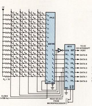
Fig 6 Keyboard encoder circuit diagram. FPLS scans switch array in 4 rows of 15 switches. Once switch row is selected by low level indication, FPLS seeks low level within that row to locate depressed key. At right, 8212 provides holding register function for microprocessor interface
