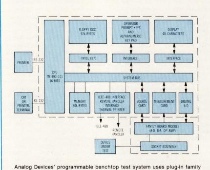
Analog Devices' programmable benchtop test system uses plug-in family board modules to provide capability for parametric testing on A-D or D-A converters as well as linear operational amplifiers. Integral 16-bit microprocessor and memory allow unit to perform statistical analysis on test results. IEEE-488 interface provides communications capability
