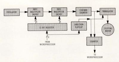
Fig 7 Stepping motor drive. Unlike dc servo in Fig 6, no encoder is coupled to shaft. However, feedback control is required to generate command frequency. Steppers also have more inherent peculiarities than do dc servos (eg, resonances)
