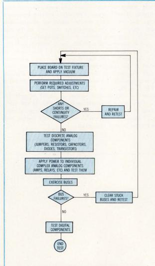
Fig 8 In-circuit testing flow chart. More common defects are checked out first. Test ends if shorts or stuck buses are encountered, since these may contaminate later portions of test
