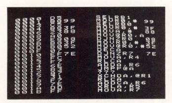
Fig 7 Program disassembly display segment. General purpose routine generates two-to-nine character mnemonic plus operands from machine instructions in program memory. Typical 8035 instructions are shown, but virtually any microprocessor instruction set is handled. Disassembly is a powerful aid to locating both software errors and program entry errors
