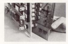
Switches may be wave soldered directly to the PC board, eliminating hand soldering and prewiring. Connectors with straight or 90° pins mate with low level and electronic switching elements in series 01, 11, 14, 21, 31, and 41 switches. They are permanently soldered to the PC board and pressed onto the switches already mounted on the panel. Low level switches are suited to current <100 A and 60 V. **EAO Switch Corp**, 255 Cherry St, Milford, CT 06460.
