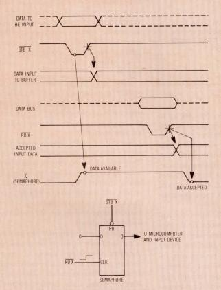
Fig 2 Conditional input with semaphore. Timing diagrams demonstrate sequence of timing signals and data transfers for microcomputer input using semaphore shown
