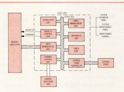
DPS-330 central processor consists of control store and channel buffering unit. Logic unit is formed of eight separate asynchronous units grouped together. Logic unit can execute up to five microinstructions in parallel in total of 315 ns
