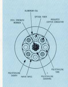
Fig 1 Cross section, optical fiber cable. Fibers are protected by loose tube rather than by tight buffer coating per BICC fiber packaging technique. This protects against fiber surface damage during cabling, and in conjunction with central strength member, isolates fibers from forces encountered during installation. Resulting cable is very stable and relatively unaffected by handling or changes in temperature
