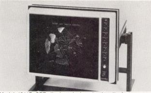
Model 1311B CRT display, designed primarily for use as a graphics computer peripheral, has resolution of 24 lines/cm at center screen with minimum corner defocusing. Using a 14" (35-cm) diag screen, unit includes high speed deflection circuits, fast rise time Z-axis amplifier, and regulated power supplies.
