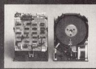
Use micro-Winchester with a minifloopy. Get Winchester's faster access time and data rate. Average access time is 170 milliseconds, almost twice as fast as the minifloppy's 298 milliseconds. Data rate? In one second, the micro-Winchester transfers five megabits compared to the minifloppy's ½ of a megabit. Save your minifloppy for low-cost backup and system I/O.
