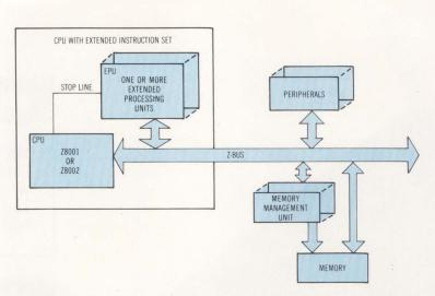
System configuration shows Zilog's Z8000 CPU employing one or more extended processing units to handle time consuming CPU tasks more efficiently
