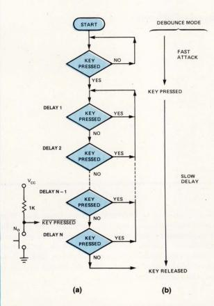
Fig 2 Scanned key (a) and sampling debounce algorithm (b). Each key acts as contact to ground, pulled up through resistor to  $V_{\rm cc}$ , producing encoded zero output when closed. Fast attack detects closure in one sampling period. Slow delay takes several samples to determine that key was released
