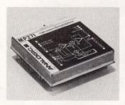
0.005%, and pedestal variation of ±0.002% max, ±0.003% linearity, is suited for use in data acquisition systems with sampling rates up to 300 kHz and resolutions up to 16 bits. Low hold mode feedthrough significantly increases system throughput by allowing the A-D conversion time to over-
