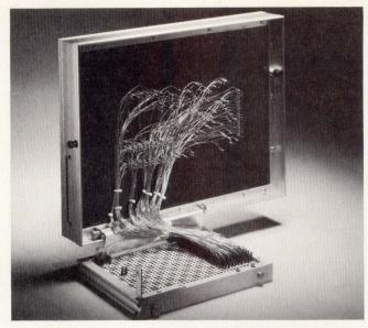
Fig 4 Test fixture showing wiring to plugboard. Connections between probe and plugboard pins can be wired at random. System software maps circuit board nodes as operator contacts them with probe
