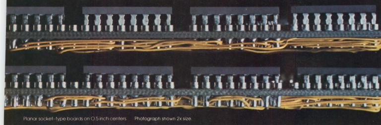
Augat's Planar stitch-wire concept is unique. This patented, high-speed, low-cost system reduces the substantial engineering time of complete circuit card
