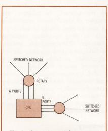
Fig 1 Common carrier system configuration. Multi-line rotary exchanges allow large numbers of users to contend for computer ports through its switched network
