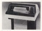
consumption, and a minimum of mechanical parts which permit cooler operation and increased reliability. In addition, high energy magnets, custom IC hammer drivers, and steel band font carrier contribute to performance. The easily replaced steel
