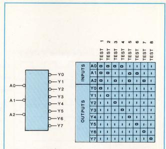
Fig 1 Classical approach to testing 3- to 8-line encoder. Truth table values are applied to inputs and corresponding output values measured. Testing all possible states requires eight separate tests. Writing code to generate distinct input states takes time and resulting test programs are unwieldy, especially for testing complex devices that incorporate sequential logic
