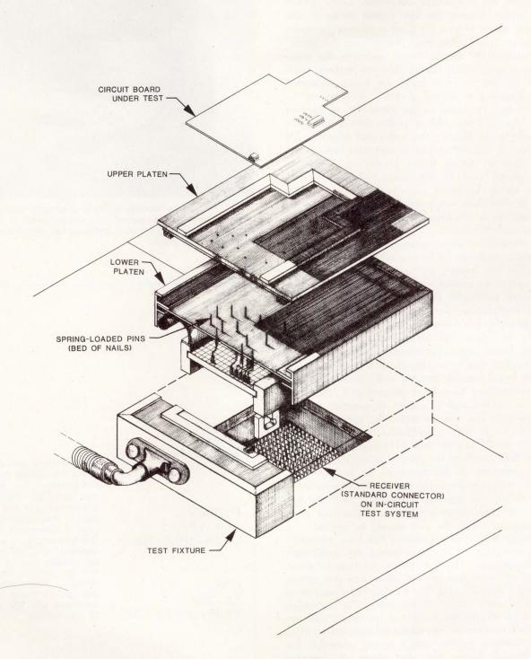
Fig 3 Test fixture, exploded view. Receiver or other standard connector joins test fixture to numbered test system nodes. Fixture pins contact circuit board nodes when vacuum is applied to test fixture
