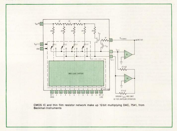
The series 7541 12-bit multiplying digital to analog converter from Beckman Instruments Inc, 2500 Harbor Blvd, Fullerton, CA 92634, consists of a CMOS integrated circuit and a thin film R-2R ladder network combined in an 18-pin side-brazed ceramic DIP. This DAC is a second-source pin for pin replacement for the AD7541 from Analog Devices.
