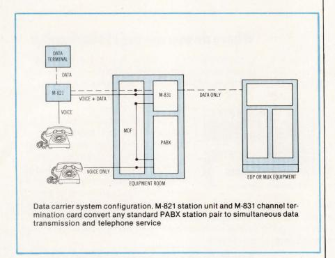
Data carrier system DCS-2B uses high frequency carrier techniques to add a data communications link to an existing PABX telephone pair. The derived point to point link is capable of 0 to 9600-bit/s full duplex asynchronous operation, and does not interfere with normal telephone service. Need for RS-232-C cable, additional twisted pair, or short haul modems is eliminated, according to the system developer, Teltone Corp, 10801 120th Ave NE, Kirkland, WA 98033.
