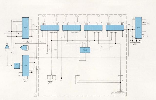
Fig 2 Logic circuit implementation. Fixed microcycle bit-slice design (within broken lines) is limited to use of 100-ns IDM2901A components, allowing general multiply execution time no lower than 124 ns. Expanded diagram adds one or more MUXs, external exclusive-OR gate, and simple flipflop (74S74). This allows faster bit-slice components (IDM2901A-2), and execution time for same operation is reduced to 79 ns
