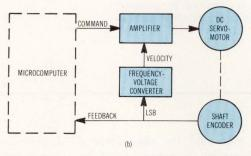
Fig 6 Typical dc servo control system. Feedback control of position servos (a) is implemented partly in software (elements within dashed box) and partly in hardware. Inner velocity feedback control loop is entirely hardware. Tachometer can be eliminated (b) by frequency to voltage converter driven from shaft encoder least significant bit
