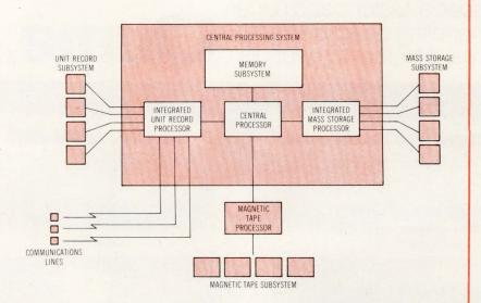
Processing capability of Honeywell's Level 64 DPS-330 is distributed between the central processor subsystem and up to seven peripheral processors, which operate asynchronously with CPU and with each other. CPU subsystem consists of memory subsystem and CPU. Each class of peripheral devices is controlled directly by its own peripheral processor
