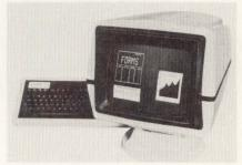
ASCII and APL versions of the concept 520 series, with either 1 or 4 full pages of display memory, emulate std features of the DEC VT-52, including cursor control, reverse line feed, clear functions, and alternate keypad mode. All 4 members are compatible with DEC software. Other features are windowing, programmable function keys, business graphics, multiple char sets, and multiple I/O ports. Human Designed Systems, Inc, 3700 Market St, Philadelphia, PA 19104. Circle 260 on Inquiry Card
