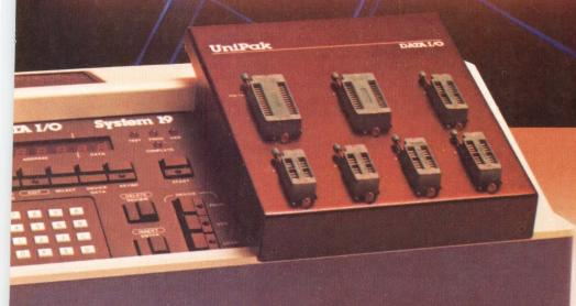
Our new System 19/UniPak lets you program most MOS and bipolar PROM'S from AMD, Fairchild, Harris, Intel, MMI, Motorola, National, Raytheon, Signetics and Texas Instruments. UniPak's software assembles the programming algorithm and selects the correct socket for 16, 18, 20, 24 and 28-pin PROMS.
