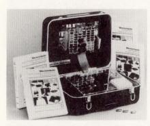
Integrated Computer Systems' kit provides hardware in portable case together with self-study manuals to solve organization's training needs for microcomputer software, hardware, and realtime interfacing
