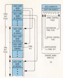
Fig 6 Breakpoint status change table entry format. General purpose routine driven by this table parses operator input to identify both microprocessor register and new data to be placed in register. Entry triplet (a) consists of ASCII character and pointer to either next key subfield or register destination. Final key triplet (b) terminates entry and supplies destination page address
