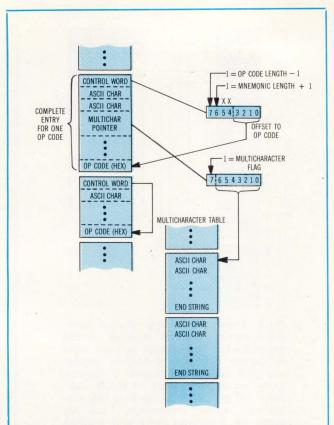
Fig 8 Operation code table entry format. Multiple byte entries headed by control words specify offset to start of hexadecimal op code. Control word may show increment of mnemonic length or decrement of op code length. Character entries are either single ASCII codes or pointers into multiple character table
