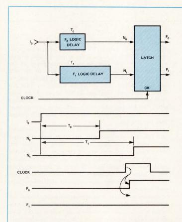
Fig 5 State machine setup time violation. Signal on I affects two different outputs,  $F_{\rm o}$  and  $F_{\rm 1}.$  When  $I_{\rm 0}$  is asserted high, both  $F_{\rm o}$  and  $F_{\rm 1}$  are to assume high next output state. However, since  $F_{\rm 1}$  has propagation path longer than  $F_{\rm o}$  and requires full setup time, any setup time violation results in next state of  $(F_{\rm 1},\,F_{\rm o})=(0,\,1)$  instead of correct output,  $(F_{\rm 1},\,F_{\rm o})=(1,\,1)$
