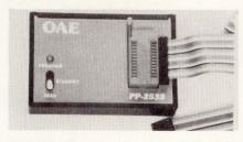
PP-2532 for the 4k x 8, 5-V only, TMS 2532 EPROM converts a P/ROM socket to a table top programmer using a 4' (1-m) flat ribbon cable that connects this device to any P/ROM socket via a 24-pin plug. With the P/ROM socket interface, data are sent over the 8 lower address lines to program the P/ROM. Each tabletop unit contains an internal dc to dc switching regulator and zero insertion force socket. Oliver Advanced Engineering, Inc, 676 W Wilson Ave, Glendale, CA 91203.
