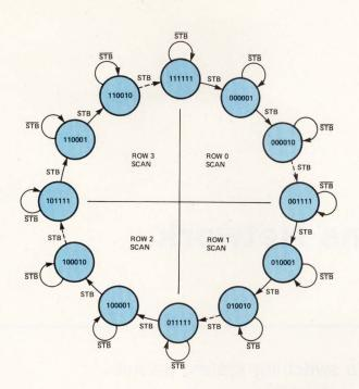
Fig 8 Key scanning state diagram. Modulo 60 counter forms sequence required to monitor all 60 keys. At each state, different key is sampled for change of state. When monitored key is depressed, KEY STROBE line (STB) is asserted low after next clock pulse, thereby stopping key scanning count, which signals unique code for each depressed key
