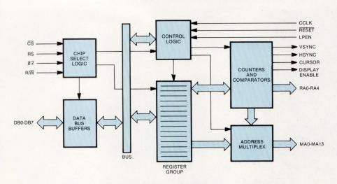
Fig 1 Internal block diagram of SY6545 CRT controller. Register group contains all programmable parameters to fully define video display formats. Counters and comparators are employed extensively to generate scan address and video signals
