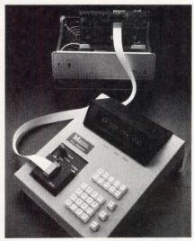
ROSI ROM simulation module located in lower left corner of International Microsystems' 1010 programmer debugs programs before they are committed to P/ROM. Module is complete with 24-pin cable and standard socket adapter
