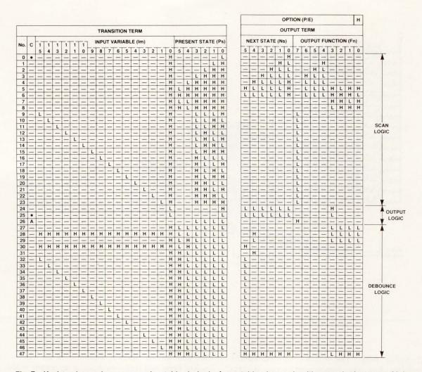
Fig 7 Keyboard encoder programming table. In logic form, table shows algorithm required to scan 60 keys. Lines 0-8 reflect cyclic key scanning count. Lines 9-23 map states into particular key. Lines 24-25 complete output key code. Line 26 completes output cycle. Remaining lines reflect debounce logic
