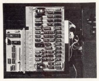
Fig 1 Universal interface. Simple 8035 satellite plugs into edge connector at lower left. Ribbon cable at right attaches to host computer. Edge connector at upper left allows expansion of multiplexed program RAM. Satellite may be replaced by ribbon cable connection to application system ROM socket
