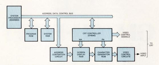
Fig 2 Microprocessor-based CRT system. CRT controller addresses both screen display RAM and character generator ROM. Sizes of RAM and ROM needed depend upon number of characters to be displayed, character font, and size of character set. Address contention circuits permit processor to gain access to screen display RAM in order to read or change its contents
