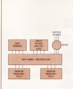
Fig 2 Dedicated channels and contention hardware. More economical than common carrier system, however, interprocessor connections are difficult and number of ports and terminals are limited by hardware
