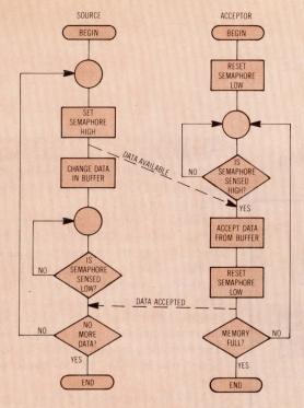
Fig 1 Flowcharts for source and acceptor. Communication between source and acceptor is shown by dotted lines, which represent two output states of single semaphore
