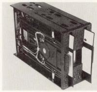
Handling 2 independent 5.25" (13.33-cm) diskettes while maintaining size and interface compatibility with other single 5.25" drives, "DAM" floppy model A-40 provides single-sided, dual-density recording on 40 tracks of each diskette. Track to track access time of 12 ms produces a random average seek time of 170 ms. Unformatted storage is 256k bytes/diskette or 512k bytes/drive. **T and E Engineering, Inc,** 1010 W 190th St, Gardena, CA 90248. Circle 217 on Inquiry Card
