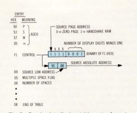
Fig 5 Breakpoint display table entry format. General purpose routine driven by table entries displays status of virtually any microprocessor. ASCII "=" preceeds reference to data outside table. Subsequent entries serve to locate, adjust, and format data
