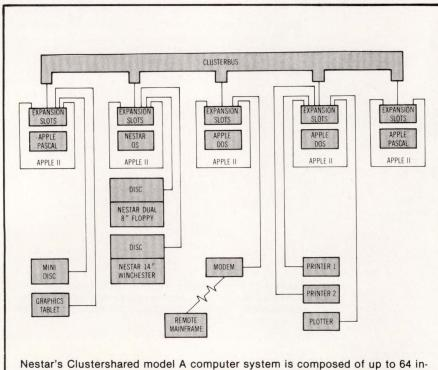
Nestar's Clustershared model A computer system is composed of up to 64 independent Apple II microcomputers in a local communications resource sharing network. System uses one dedicated microcomputer as central mass storage manager which connects with all user stations through ClusterBus
