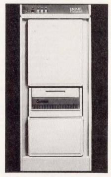
Configured and supported for implementation of dedicated or distributed processing systems in multiple locations and providing the large memory space necessary to run mainframe programs, the 32-bit PRIME 150 boosts throughput by use of microcode and high speed cache memory
