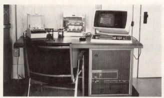
Fig 1 Micro-Coal 1 control console. MicroNova microcomputer is in cabinet at right, just above dual floppy disc drive. Interfacing circuitry and audio alarm are in upper section of cabinet. CRT displays main menu, allowing operator to choose laboratory functions. Balance at left corner of desk weighs samples of up to 30 g at accuracy to 0.0001 g. Pedal switch to left of CRT terminal strobes microcomputer for reading balance
