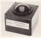
ment of the cursor with 1 hand; 2 incremental encoders sense the movement as the operator rotates the ball. Incremental digital output of the encoders represents direction and magnitude of rotation in each axis. Operation is over a 0 to 55 °C range, with power input of 5 Vdc ±5% at 200 mA max to TTL
