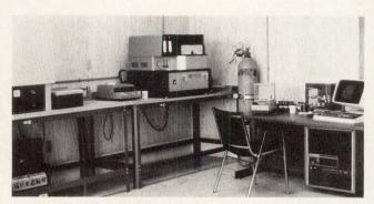
Fig 2 View of laboratory. Components (from right to left) include control console, sulfur analyzer and controller, printer, and moisture oven
