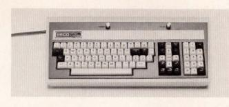
Fig 7 Keyboard variation for hotel system. Volume control adjusts level of clicks that simulate typewriter sounds. Multiple transmit keys reduce hand travel required to transmit data
