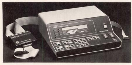
Host computer acts as multiprocessor development system with addition of Millennium Systems Series 2000 emulator that uses discrete microprocessor cards
