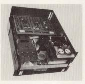
The 21M-byte HD-11—a Shugart industry standard SA4000 Winchester drive with optional 15M-byte DEI cartridge tape backup module—solves data loss if the sealed disc is ever unrecoverable. This packaging of a disc and tape drive in the same chassis is a method of fail-safing disc drives or allowing large offline
