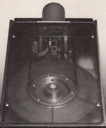
**Proven Reliability.** BASF, because of its experience in both magnetic media and drives, is highly qualified to develop drives using reliable 3350 Winchester technology. BASF 6170 drives have a 10,000 hour MTBF and require no scheduled maintenance or operator intervention.
