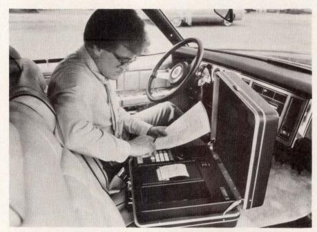
Norand's Route Commander combines data collection terminal, data storage capacity, and printer with processing and telecommunications capabilities in portable unit to extend benefits of computer data processing into distribution industry
