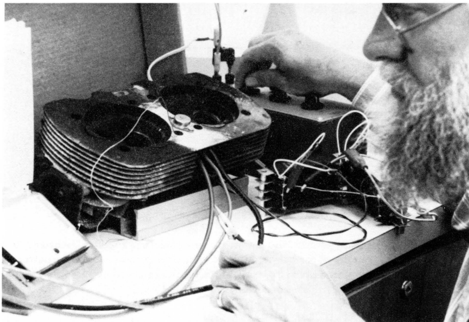
Figure 7.4. When using high-power amplifiers, there are certain problems you just never have if you use a big-enough heat sink. This heat sink's thermal resistance is lower than 0.5\text{ }^{\circ}\text{C/W} . (Photo copyright Peggi Willis.)
