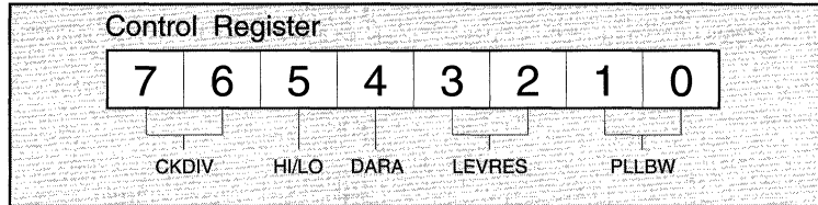
Figure 17 - The Control Register
